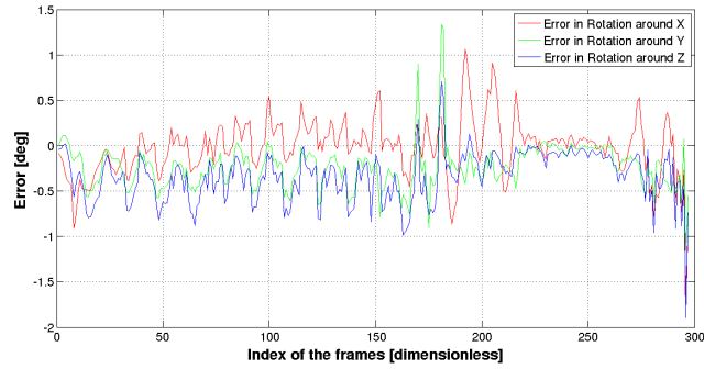
(c) Error in rotations around X, Y, and Z for images with motion blur and noise (60 fps-blur dataset)
