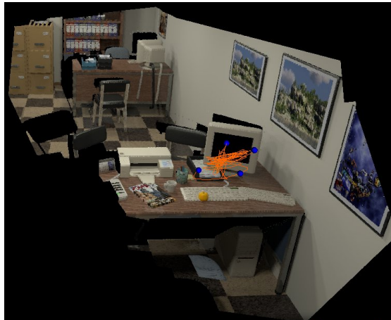
Figure 2.10: Dense Map built using depth maps of keyframes. The trajectory is drawn in orange and keyframes are blue spheres.
