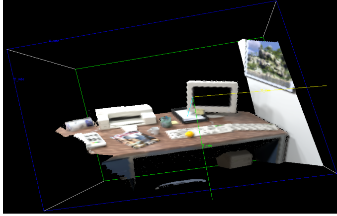
Figure 2.12: 3D reconstruction resulting from fusing synthetic depth maps and color of the scene, from the estimated camera pose.
