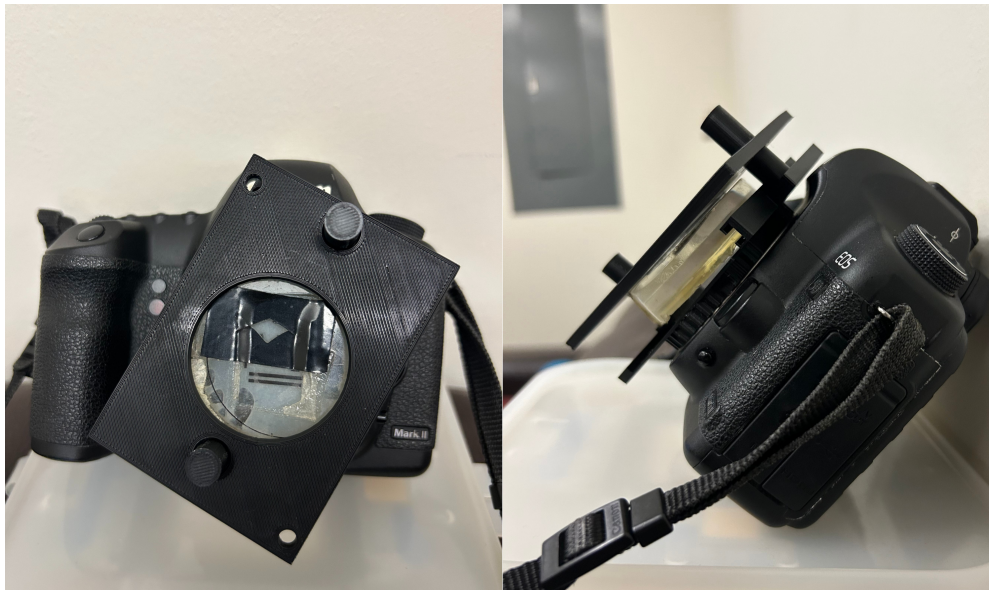
Figure 3.7: 3D print holder fitting into the camera.
