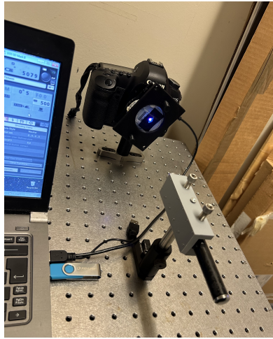
Figure 3.4: Set up for the laser pointers aligned to the camera at a 15,24 cm distance.
