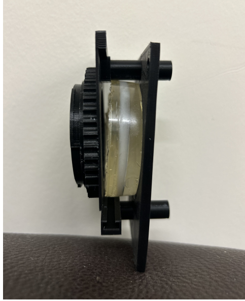
Figure 3.8: Image of the sample not completely parallel to the holder.
