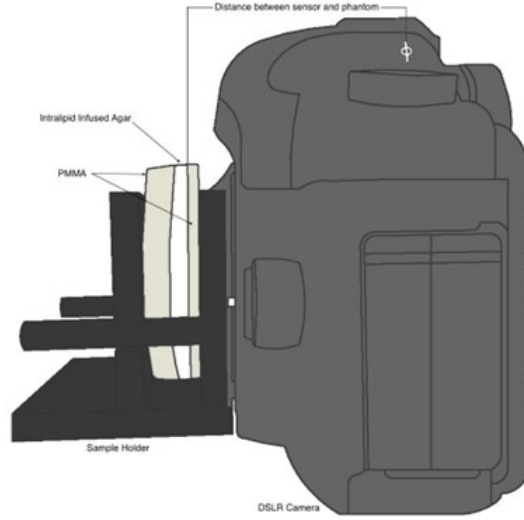
Figure 3.2: Schematic scattering phantom and camera arrangement [3].
