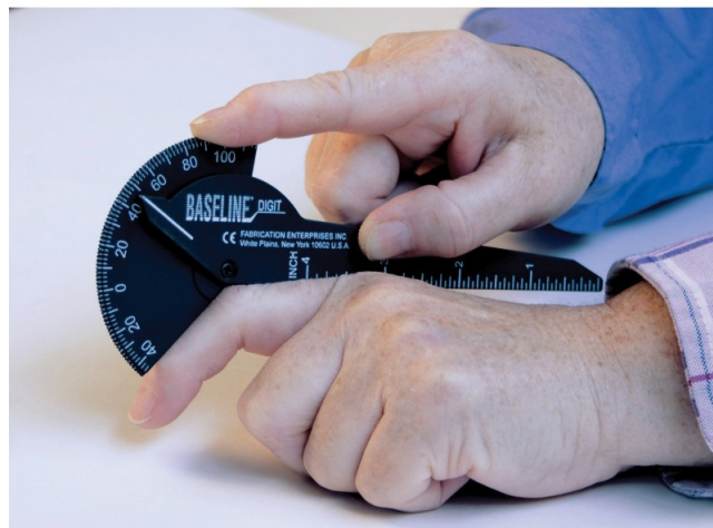
FIGURE 4.3: The goniometer is used to measured the angles in different grips positions. Source: FisioStore.it
