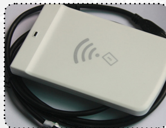
Imagen 34, Lector de RFID Medidas 80mm x20mm. Recuperado de: http://m.alibaba.com/product/60076750899/1M_Reading_Distance_USB_Passive_RFID/productdetail.html
