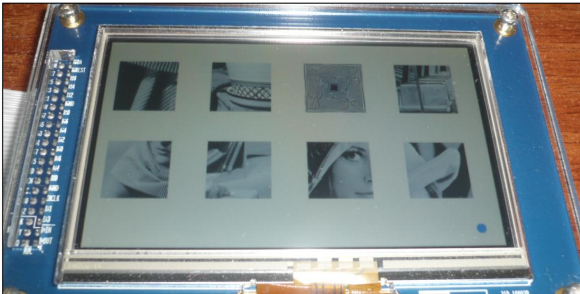
Figure 44. Thumbnails of the images available in the SD-Card for Bandelet processing.
