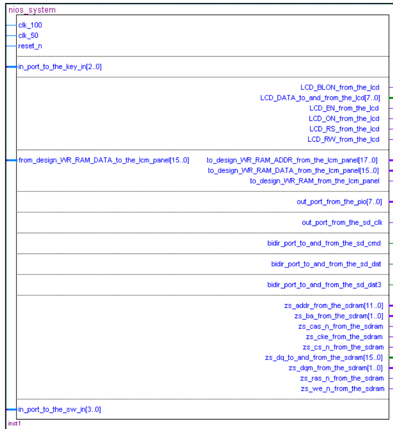
Figure 20. Schematic capture symbol generated by SoPC Builder for JPEG File Viewer.
