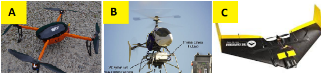
Figure 2.7.: Common aerial platforms used in agriculture contexts. (A) multirotor, (B) helicopter, (C) fixed-wing.
