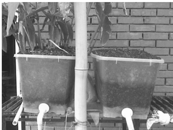
Figure 2. Pilot-scale subsurface constructed wetlands
