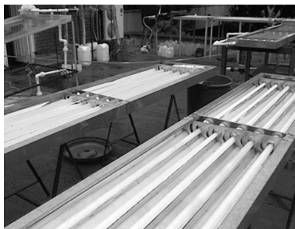
Figure 1. Solar CPC reactors (Universidad del Valle, Cali-Colombia)
