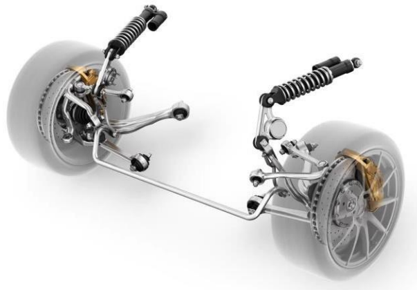
Fig. 1. Sistema de suspensión multi-link delantera del Mercedes-Benz SLS AMG E-Cell supercar. Tomada de: https://newatlas.com/mercedes-sls-amg-e-cell/21778/
