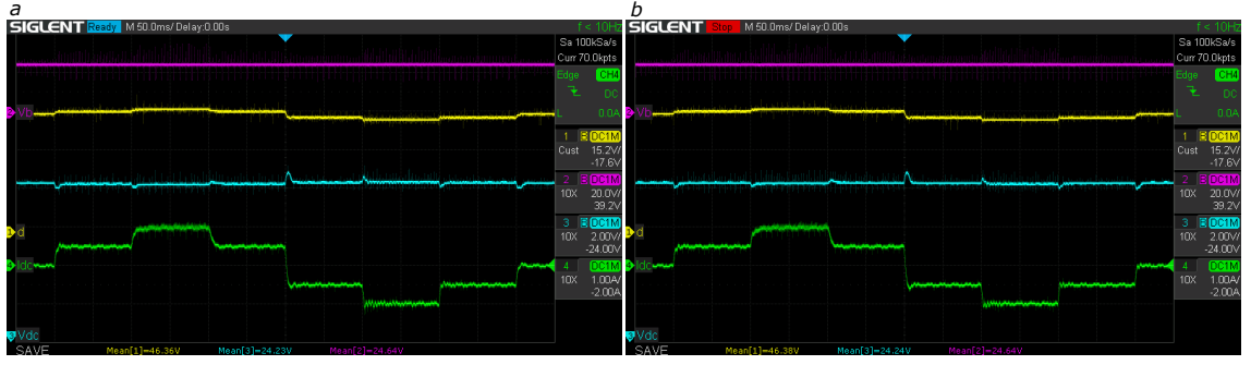
Figure 5.8: Bus regulation with V_b = 24\text{ V} and reference V_{dc_{ref}} = 24\text{ V} (unitary gain mode) using Adaptive LQG a) with Lookup-table, b) with polynomial interpolation. Magenta: battery voltage V_b , yellow: duty cycle d , cyan: bus voltage V_{dc} , green: bus current i_o
