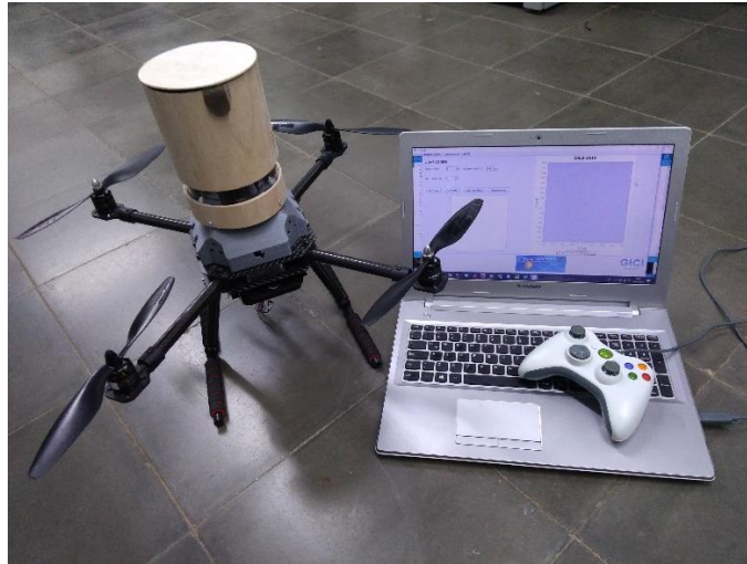
Figure 4.1. Physical configuration for the Flight Controller + GALS GUI.
