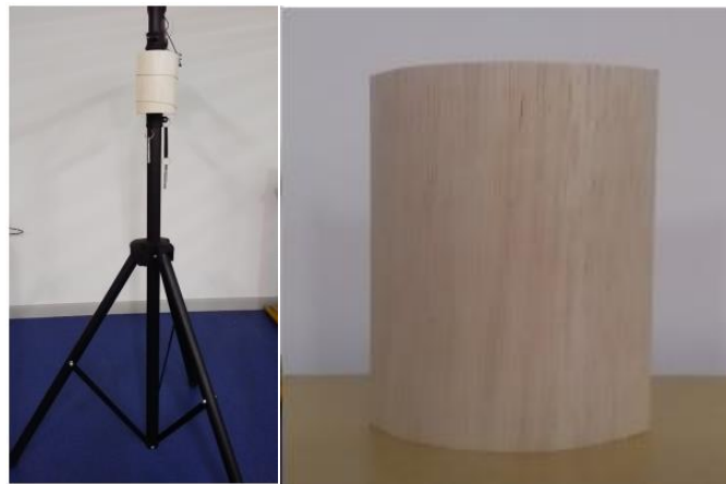
Figure 3.13. Cylinder used to perform identification tests with LiDAR.
