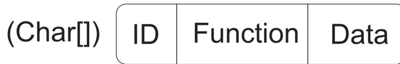
Figure 3.32. Communication protocol between the Ground Station and the Smartphone.
