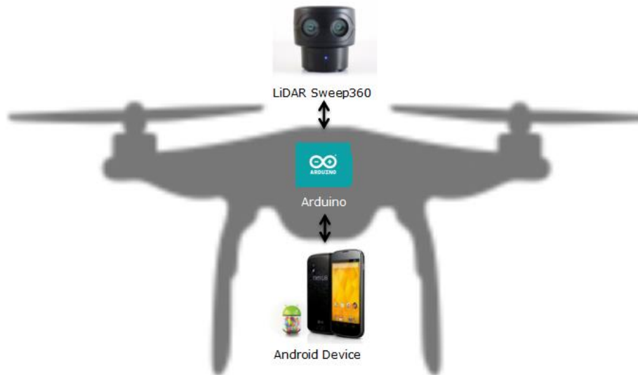
Figure 1.3. Communication lines between sensor and processing devices on each UAV [17][18][19][20].
