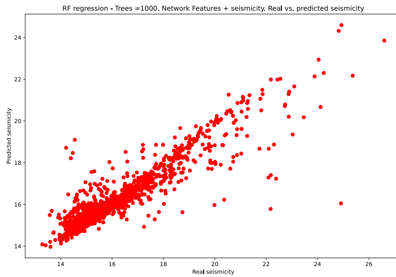
Figure 57: Random Forest Regression of seismicity of the next 20 events using network and catalog features and 3D networks with 50 events windows.
