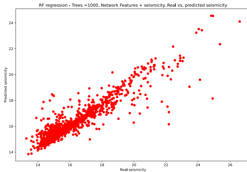
Figure 56: Random Forest Regression of seismicity of the next 20 events using network features and 2D networks with 50 events windows.
